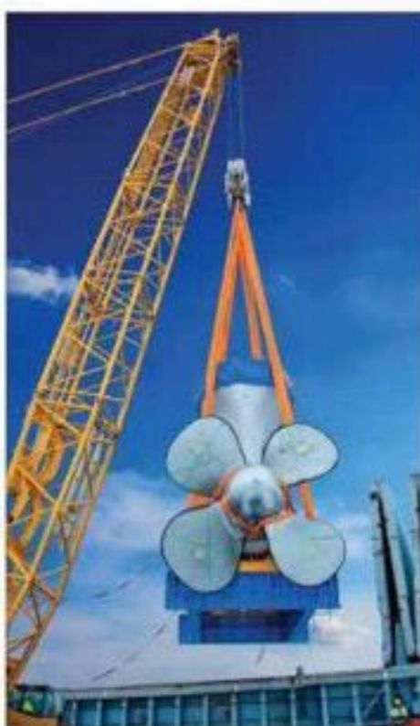
Picture: Lifting of a 30St Azipod unit with Forankra 100t roundslings.
